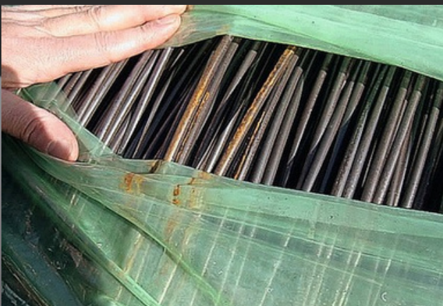
Metal after transport without VCI protection
