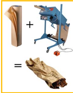
The PadPak® converting process
